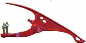
This fully adjustable crop lifter is designed to fit combine floating cutterbars with 11/2" cut stub It is equipped with a set screw height quards. adjustment, non-clogging spring action joint, and is double-bolted to the cutterbar. 4S crop lifters are constructed of ductile iron for strength and durability. They are equipped with high strength yellow zinc plated fasteners.
