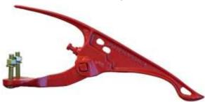
This fully adjustable crop lifter is designed to fit combine floating cutterbars with  $1\frac{1}{2}$ " cut stub guards. It is equipped with a set screw height adjustment, non-clogging spring action joint, and is double-bolted to the cutterbar. 4S crop lifters are constructed of ductile iron for strength and durability. They are equipped with high strength yellow zinc plated fasteners.
